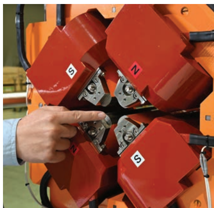
The four poles of magnets that guide electrons used to produce X-rays in SPring-8-II
