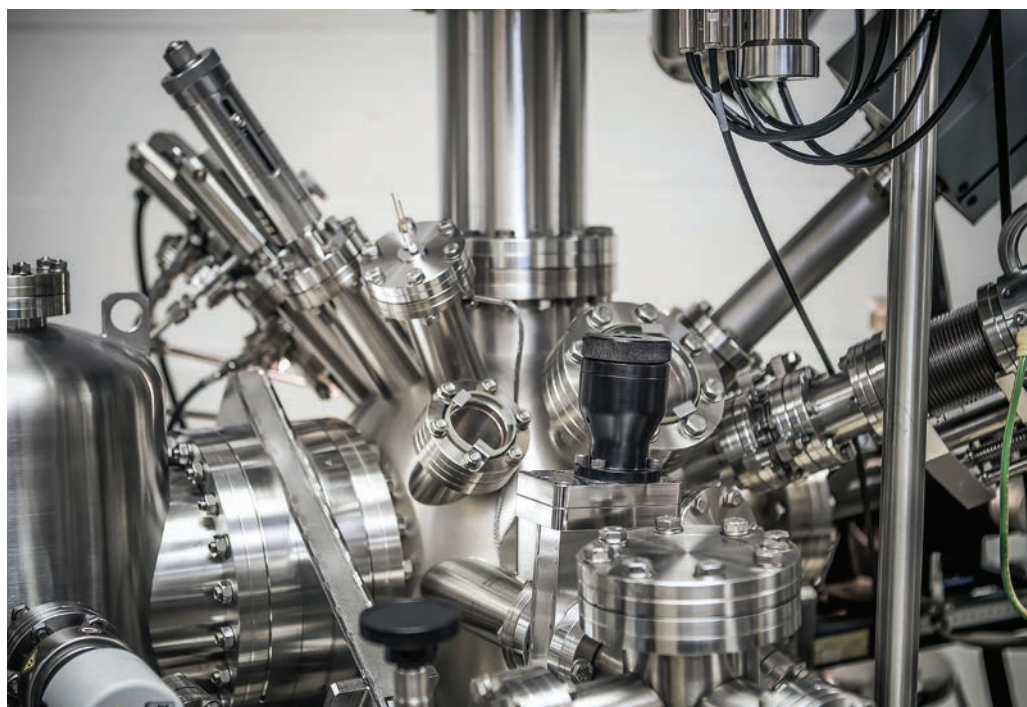
Molecular beam epitaxy systems, such as this one, are used to form highly precise thin films with multiple layers. Usually, the lattices of adjacent layers should be very similar to each other to obtain high-quality films, but RIKEN researchers have found an exception to this rule.
