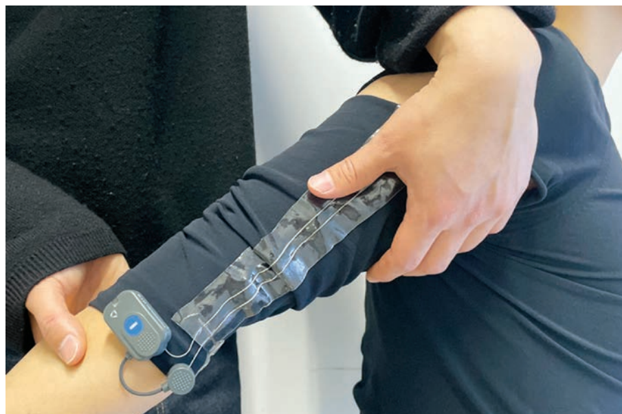
One of the wireless electromyography modules (bottom left) that is used to transmit data collected from the wearer.
