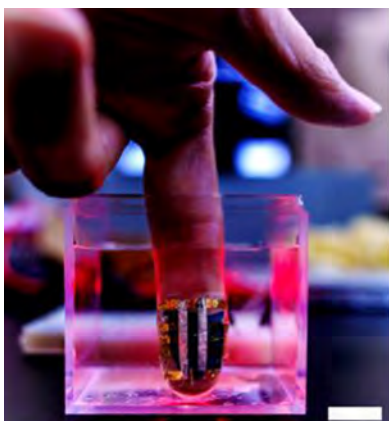
Fig.1 Photograph of organic optical sensor attached to the finger
